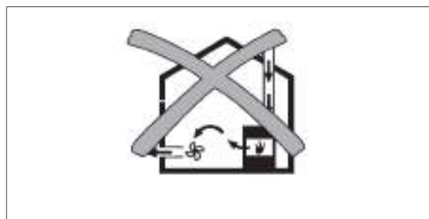
Fig. 4.1 Exhaust air installation – not permitted
